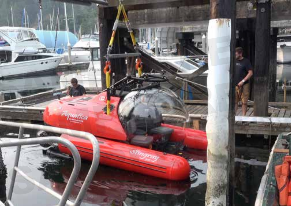
(Top) The prototype Stingray 500 three-man submersible being deployed by crane at the marina launch site close to the dive site. (Bottom) A juvenile male sixgill shark estimated at 2.0 m tl, adjacent to ballast chamber of Aquatica manned submersible (diameter of chamber 60 cm for scale). Sharks were highly attracted to metal and electrical elements of the submersible.
